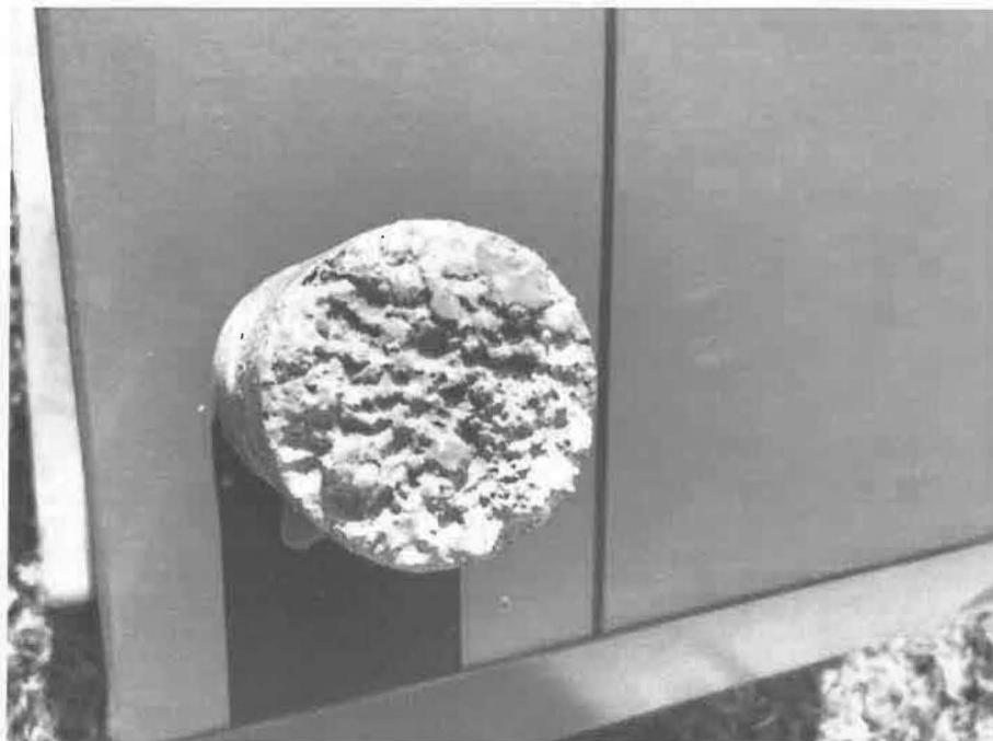
Photo 8 – Typical view of erosion in collected sample.
